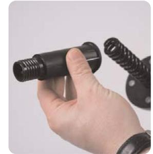
Slide the plastic insert over the pole/spring assembly. **4**
